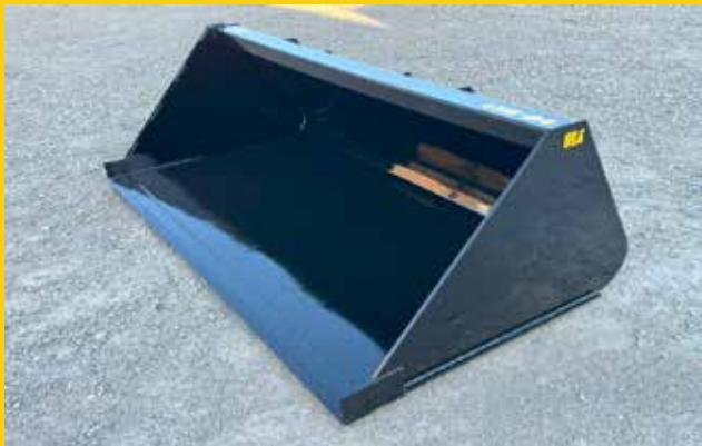
The Stinger Attachments Liquid Slurry Bucket is ideal for liquid slurry type products. This is an extremely high volume bucket that is designed to carry a full load of liquid slurry. The 60 degree back angle allows for increased rollback, which enables the operator to level the bucket edge for maximized liquid carrying capacity. This bucket is offered with multiple mount options
